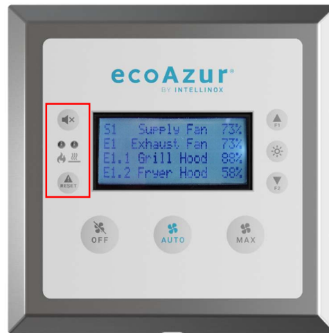
Figure 12 - V6KP-100 SILENCE AND RESET KEYS
